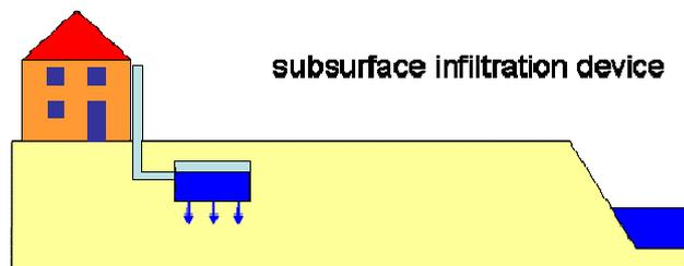
(soakaways). Maintenance in case of clogging or pollution is difficult and often only effective in a limited way. High groundwater tables in some parts of the Netherlands limit the application of these systems.
